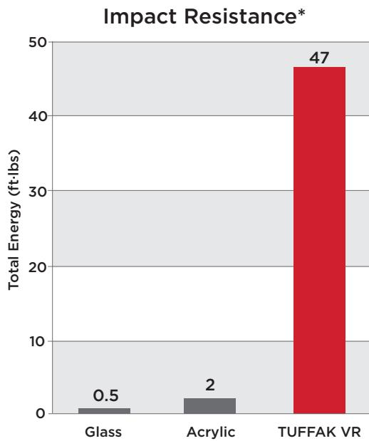
\*Instrumented Impact per ASTM D 3763, sample thickness 0.125" nominal
