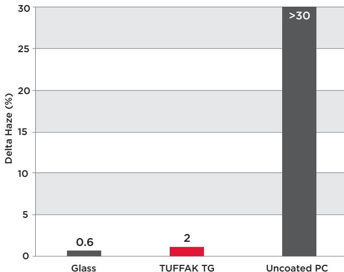
\*Taber Abrasion per ASTM D 1044, 100 cycles using CS-10F wheels at 500 g load
