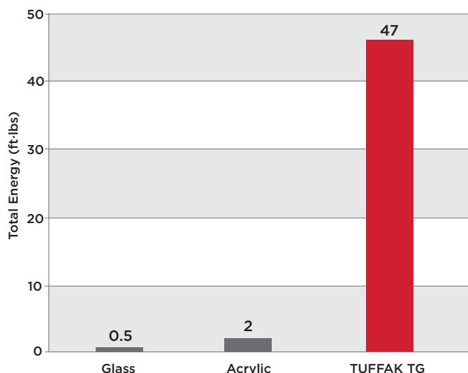
\*Instrumented Impact per ASTM D 3763, sample thickness is 0.125" nominal
