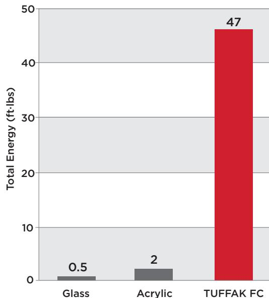
\*Instrumented Impact per ASTM D 3763,
