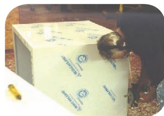
Seams are routed to leave a smooth, clean joint
