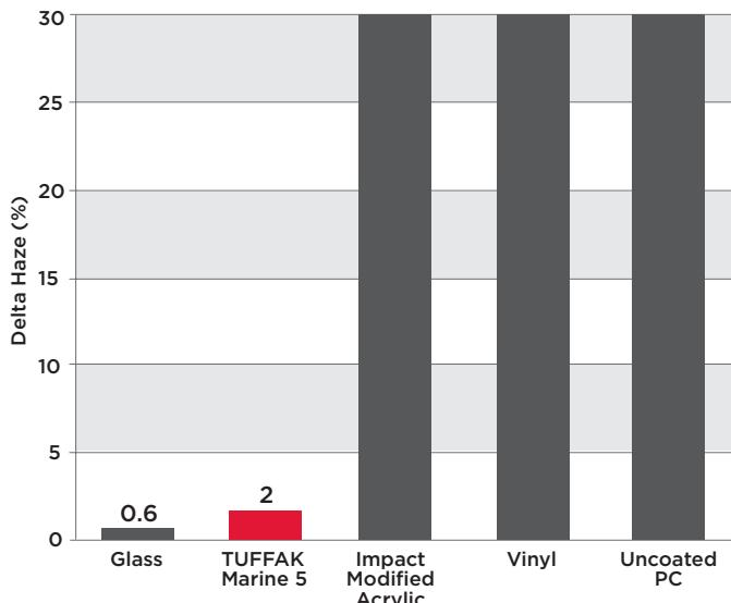
\*Taber Abrasion per ASTM D 1044, 100 cycles, CS-10F wheels at 500 g load
