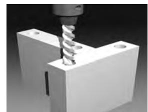
The minimum distance from the edge should be 2 times the hole diameter. In an effort to reduce heat build up during drilling of thicker Palight sheets, it may be necessary to periodically remove the drill bit from the Palight material.
