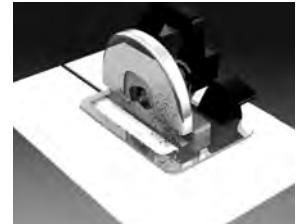
For Palight sheets 3 mm and thicker, carbide-tipped, triple chip, ground type circular saws can be used.
