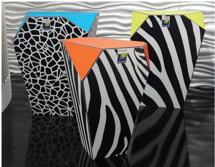
Using a combination of digital printing, v-groove cutting, and cold-formed bending techniques, Palboard was shaped into these unique trade show display podiums.
