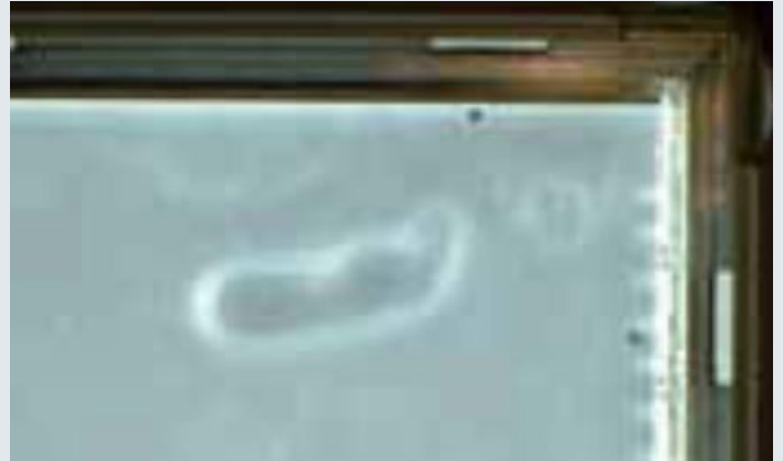
Impaired light emission caused by water droplets
